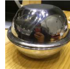
Figure 6: Stainless steel ball as a reference, made with two kitchen bowls.
