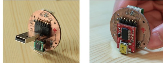
Figure 4: Exchangeable power board. The power board (left) can be replaced by a USB-serial convertor (right) for updating software on the main board.
