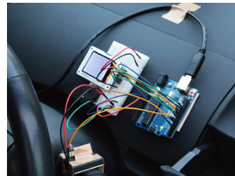
Figure 1: Problems on the prototyping in automobiles. People often have difficulty to fix devices to the car interior without spoiling the appearances.
