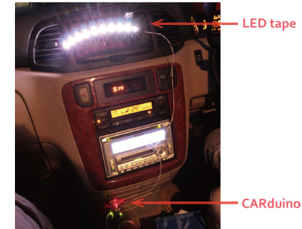
Figure 5: Interactive car illumination using the CARduino
